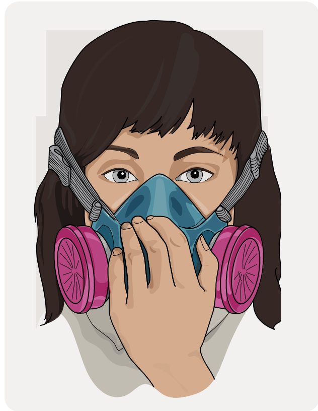
For a positive-pressure seal check, cover the exhaust valve and breathe out slightly.
